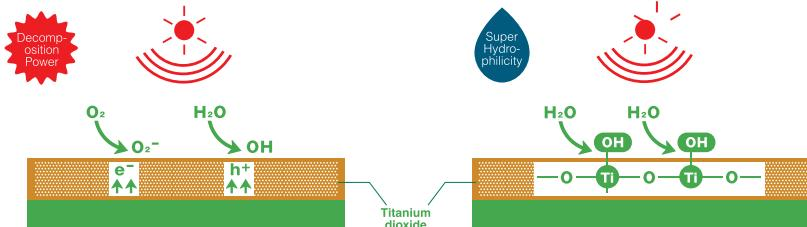
When exposed to light, titanium dioxide produces electrons ( $e^-$ ) and holes ( $h^+$ ). These react with oxygen and water ( $O_2$ ,  $H_2O$ ) in the air to produce activated oxygen ( $O_2^-$ ,  $OH$ ). This oxygen decomposes organic substances on the surface of products.
