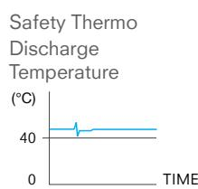
The graph shows water temperature and time. It is apparent that a conventional faucet experiences large temperature fluctuations. In contrast, the graph for SAFETY THERMO shows very little change, as temperatures are kept very steady.
