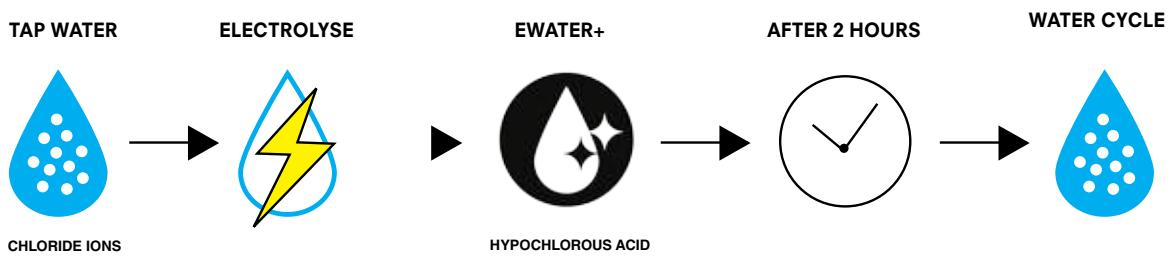
When naturally occurring chloride ions in tap water are electrolysed, they turn into hypochlorous acid, the active ingredient of ewater+. Hypochlorous acid is capable of instantly sterilising a dirty surface.
