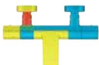
The diagram shows the temperature of the fixture after letting water run for 30 minutes, the hot water temperature set to 60° and cold set to 15°. This demonstrates how the temperatures of the main parts of the faucet – those that make most contact with the human body – are prevented from rising.
