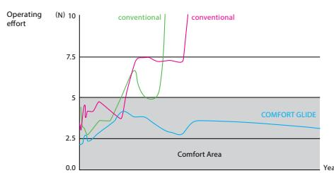
The graph shows the number of years in use, and its operating force. It is evident that comfort lasts for a long time with models featuring COMFORT GLIDE.
