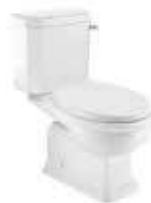
QPS-WHT-7753S250UFSPMZ Rimless Bowl With Side Flush Cistern For Coupled WC, UF Soft Close Seat Cover, Hinges, Conversion Bend, Single Flush Cistern Fitting And Fixing Accessories, Size: 420x710x810 mm, S Trap- 250 mm (With Conversion Bend) Rs. 27,700
